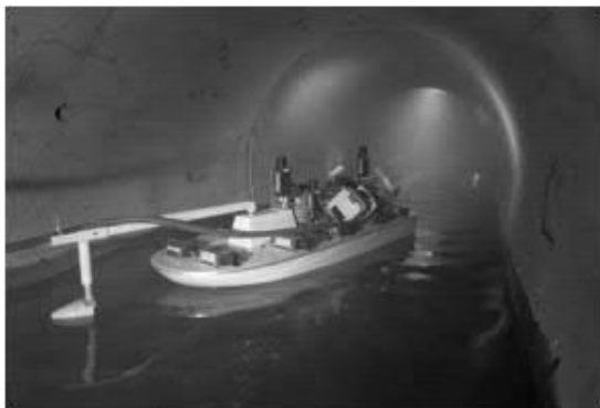
Figure 2 SEK prototype (left) and test of the SVM (right) in a real sewer
